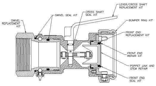
Emco Wheaton has developed a series of REPAIR KITS suitable for the field repair of the J73 Series Couplers & Adapters.
